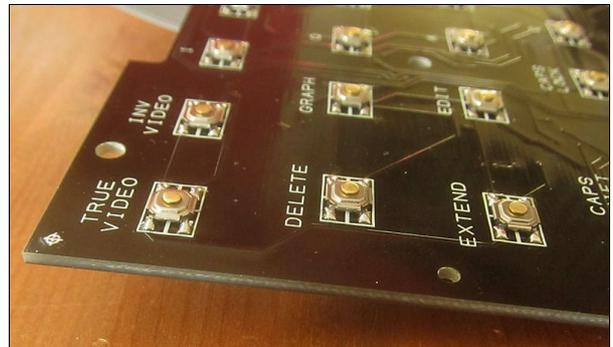
The keys to move are marked in the drawing below with an additional box around the key and an arrow indicating the direction to move. One leg of the key for the letter „Q“ should be removed or bended up which position is marked with an X. It is recommended to solder this key and the keys to move first. After all keys can be mounted centered. Precise work (position) is important for a good working keyboard.
