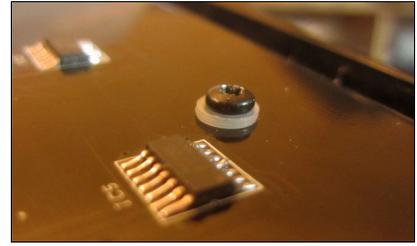
Depending on the version of ZX Spectrum+ you have to use 2 plastic washers to fill a distance of about 1mm (for the original Sinclair model with a plastic back plate). The Spectrum+ was manufactured from Samsung in licence as well with a thinner metal plate. For this model you don't use the plastic washers. The keyboard 48P-KDLX replaces keyboard membrane AND back plate.
