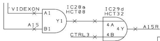
In this case the A15 mode can be activated which disables mirroring of RAM and limits the available total RAM to 32k only. CTRL3 signal fixes A15 to high which provides 32k RAM from \$4000-BFFF while mirroring \$4000-\$7FFF to \$C000-FFFF. The display file can stay in area \$4000-\$7FFF or \$8000-\$BFFF in this mode.
