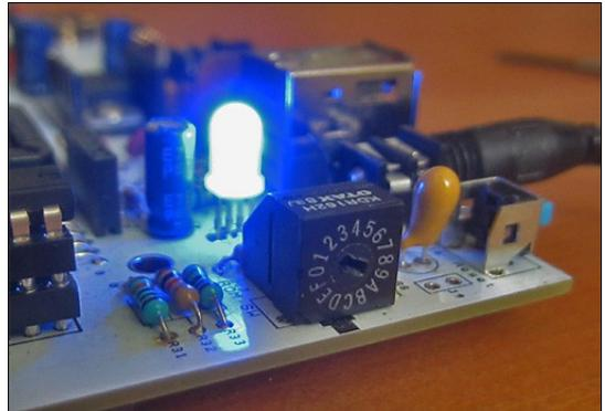
A colored LED (rgb) shows the active instance with a different color regardless if the instance is running from the manual switch or from ZXmaster control software:
