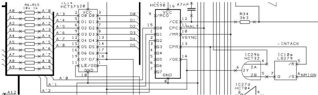
The ZXmore has no direct assignment of memory areas for HRG and UDG. The address override is activated with interrupt acknowledge cycles only which are used with UDG only but not with HRG. Plain software HRG which address the content for the video shift register with index register and refresh register do not use any interrupts.
