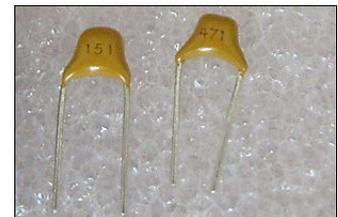
1000pF is 1nF – so a 10nF capacitor has an imprint of numerical code 103 =  $10 \cdot 10^3 = 10.000$  pF or a capacitor with 10uF is marked with 106 (10.000.000 pF). Sometimes you may see just 10u if there is enough space to print.
