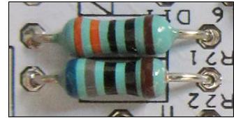
Resistors, coils, rarely some capacitors are coded with coloured rings. Depending on precision 2 or 3 rings are used to indicate the value, the forelast is the multiplier and the last one the tolerance. Every colour represents one digit.
