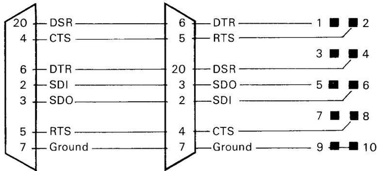
**WARNING** Do not connect the serial out lines to any circuits that are not capable of handling +12 and -12 volts. Please be advised that the serial I/O is not TTL compatible.
